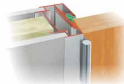
Solid panels consist of plasterboard or chipboard with a mineral wool core. The panels are held in place with the Alpha click-in system using ultra-thin plastic insert strips, and are attached to the steel supports.
